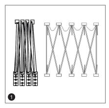
Extend frame outwards, ensuring velcro is not caught on any parts of the frame.
