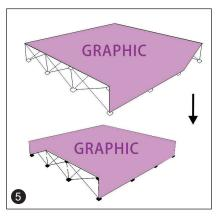
Pull end caps down to corner of frame and attach. Then attach other corner. Repeat on the opposite side.
